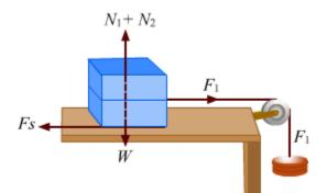
Now, the wooden blocks A and B are placed one after another. In this case, the area of contact increases, but  $W = N_1 + N_2$  remains the same. Weights are added in the pan till the blocks begin to move. Weight  $F_2$  is noted.
