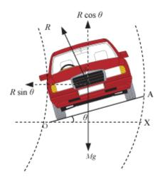
Consider a vehicle of weight Mg, moving round a curved path of radius r, with a speed v, on a road banked through angle  $\theta$ .
